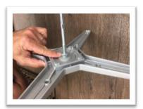
Column alignment with bottom, column should easily click in place:
