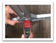
Inside tightening nut and locker washer correctly installed:
